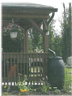
Rain barrels can also be used to collect roof runoff. Water from the barrel can be used to water plants throughout your yard and overflow can be directed into your rain garden.
